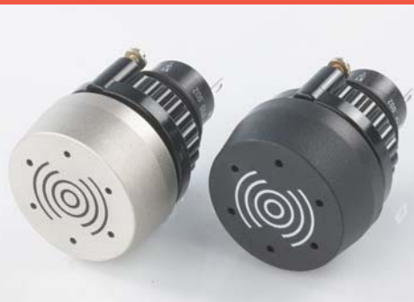
Buzzer, plastic bezel, raised, 22.5mm mounting, 24VDC, 95dB ± 8 at a distance of 0.1m
