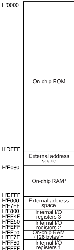
Figure 3.2 Address Map for H8S/2140B and H8S/2160B (2)
