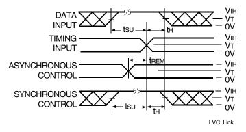
Set-up, Hold, and Release Times
