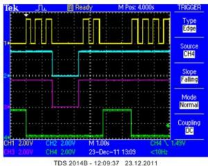
Channel 1 (yellow/top line) – pin# 8 (SMC\_INIT\_CLK) Channel 2 (light blue/2<sup>nd</sup> line) – pin# 7 (SMC\_RST\_N) Channel 3 (magenta /3<sup>rd</sup> line) – pin# 4 (SENSE) Channel 4 (green /bottom line) – pin# 2 (NMI\_GATE)
