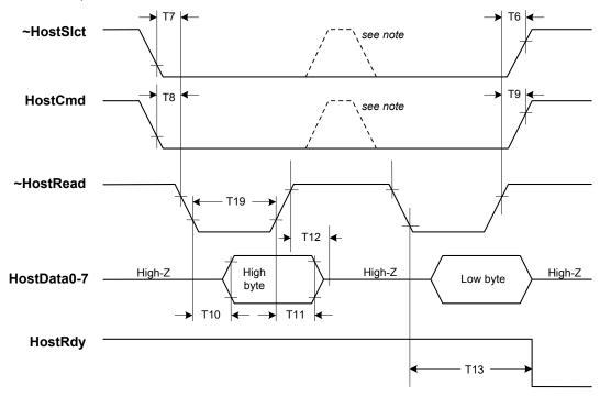
Note: If setup and hold times are met, ~HostSlct and HostCmd may be de-asserted at this
