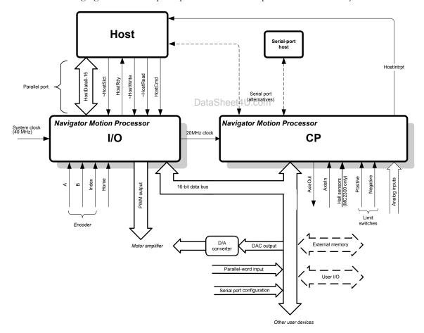
The CP chip contains the profile generator, which calculates velocity, acceleration, and position values for a trajectory; and the digital servo filter, which stabilizes the motor output signal. The filter produces one of two types of output:
