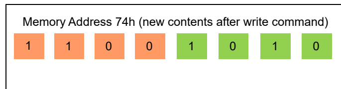
Figure 243: Example of I 2 C Byte Write Bit Masking
