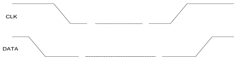
Figure 47: Timing of I 2 C START and STOP conditions
