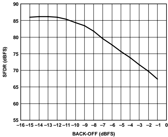
Figure 10. SFDR vs. Backoff @ AIN with f_{IN} = 70 MHz
