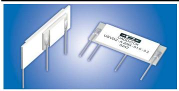
Type USVD Ultra-Precision Voltage Dividers have the very highest precision available in voltage dividers in the range of 450 Volts DC up to 2000 Volts DC. These dividers are formed by bonding together two selected Type USF Ultra-Precision Resistors. The precise selection of these high performance resistors, which form the voltage dividers, makes possible the outstanding voltage division performance. Ratio Tolerance as tight as 0.01% and Ratio TC of 2ppm/°C.
