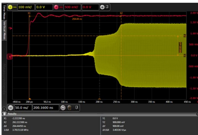
Figure 16. Switching Time Isolation to Insertion loss
