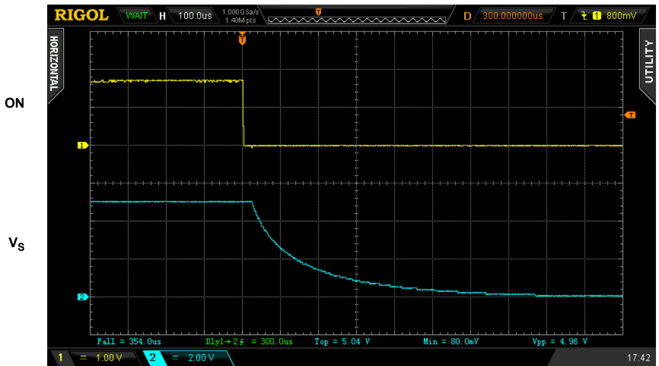
Figure 4. Typical Turn OFF operation waveform for V_{DD} = V_D = 5\text{ V} , C_{SLEW} = 4\text{ nF} , C_{LOAD} = 10\ \mu\text{F} , R_{LOAD} = 20\ \Omega
