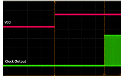
Figure 14. Startup Waveform vs. Vdd
