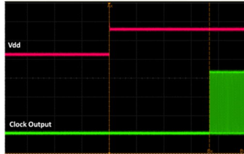
Figure 14. Startup Waveform vs. Vdd
